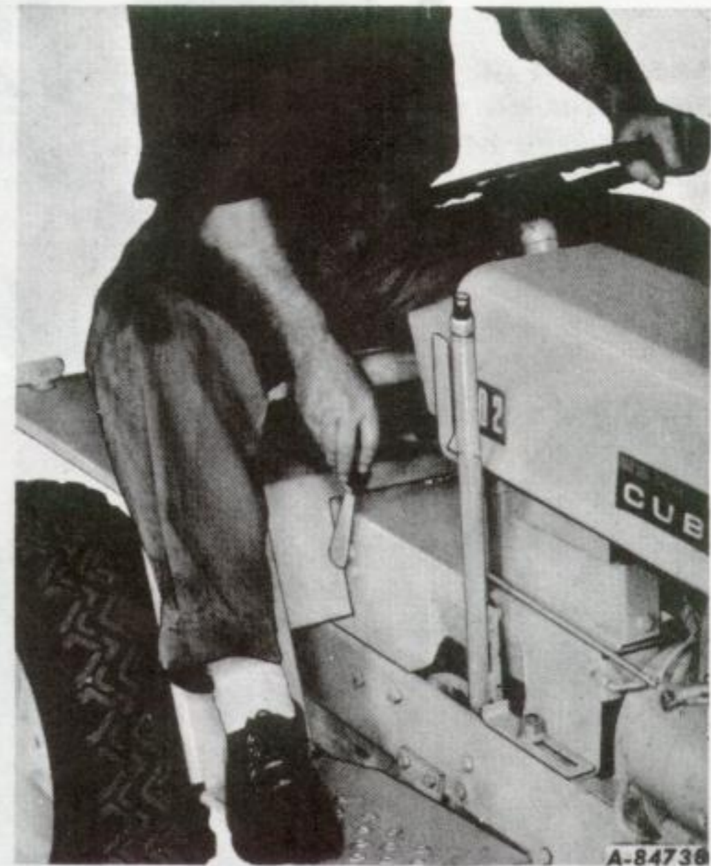
Illust. 12A Operating the Power Take-off. International Cub Cadet 102 and 122 Tractors
